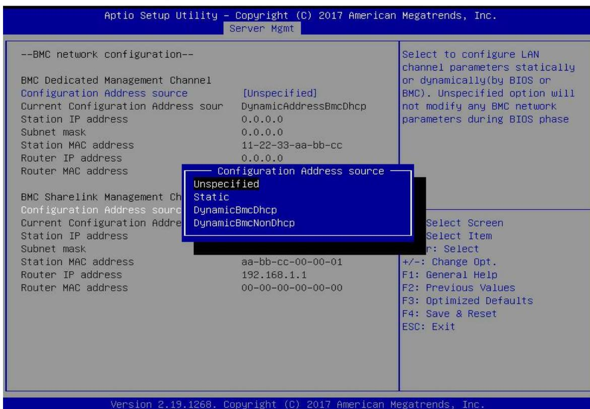
Figure 7-6 Configuring the network port network mode
